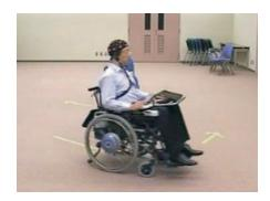
BTCC's new system fuses RIKEN's blind signal separation and space-time-frequency filtering technology to allow brain-wave analysis in as little as 125 ms, as compared to several seconds required by conventional methods. Brain-wave analysis data are displayed on a screen in real time, giving neuro-feedback to the driver for efficient operation. The system has the capacity to adjust itself to the characteristics of each individual driver, and
