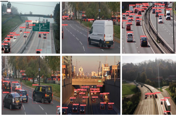
Figure 6. Some experimentations of object detection using Faster R-CNN
