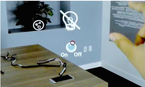
Fig. 6. Light control using HoloLens and Arduino devices [5]
