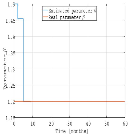
**Fig. 9.** Estimation of parameter  $\beta$  using EKF in the control loop with an initial error of 20% in parameter  $\alpha$
