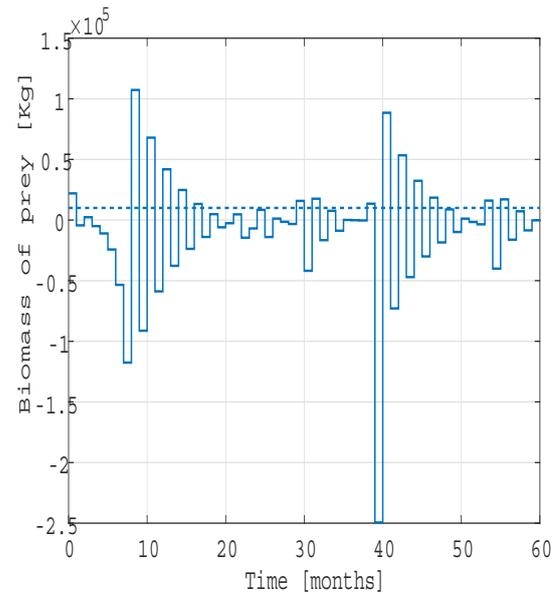
**Fig. 6.** Biomass of prey without Kalman estimator and with 20% of the error in parameter  $\alpha$
