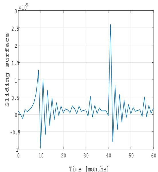
**Fig. 7.** Sliding surface without Kalman estimator and with 20% of the error in parameter  $\alpha$
