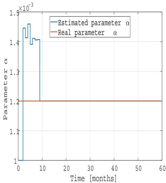
**Fig. 8.** Estimation of parameter  $\alpha$  using EKF in the control loop with an initial error of 20% in parameter  $\alpha$
