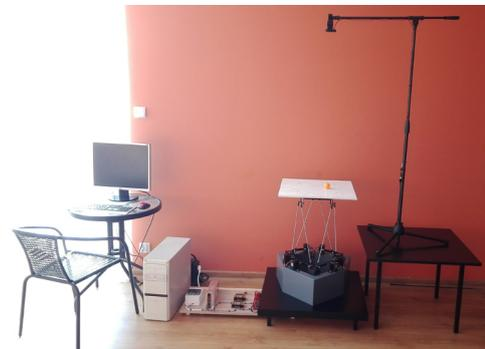
**Fig. 3.** A complete ball & plate control system research station
