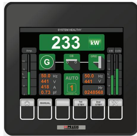
Fig. 11. TFT display for power management at a ship [43]
