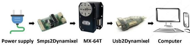
Fig. 13. Hardware setup for Motor Control
