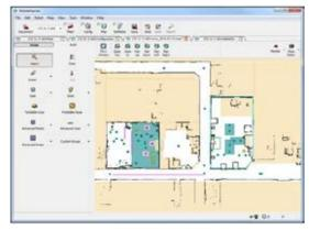
Fig. 2. The user interface of MobilePlanner – Omron [11]
