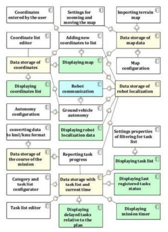
Fig. 13. Software architecture
