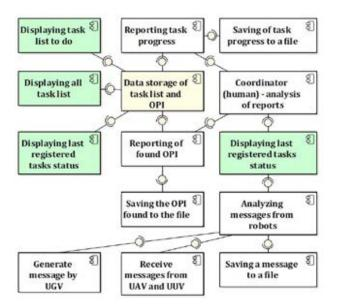
Fig. 9. Mission coordination module architecture
