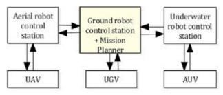
Fig. 8. Information exchange between stations and robots
