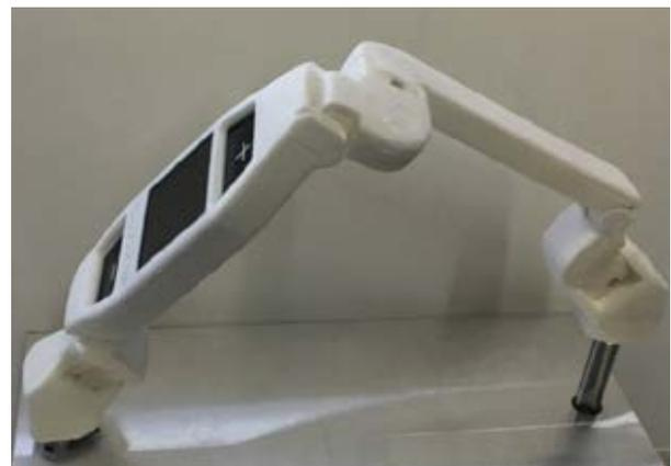
Fig. 2. Measurement arm made in 3D printing technology
