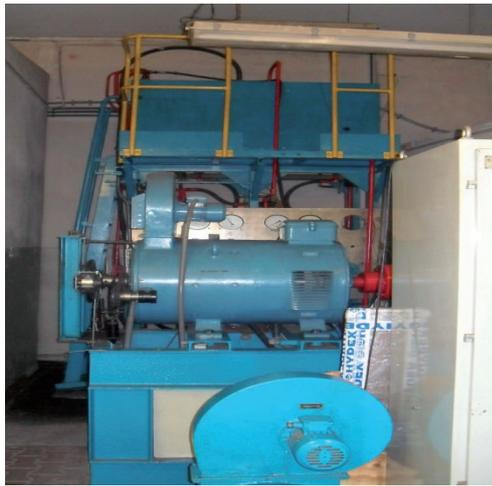
**Fig. 6. Test stand: DC drive motor, feed pump, AC motor [13]**
