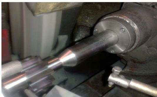
Fig. 24. The dimensions and critical deviations: 1) the beating of plugs and the lateral surface of the toothed rim 2) perpendicularity of the side surface of the tooth to the pivots (wheel rotation axis) for the detail of the gears speeding and running
