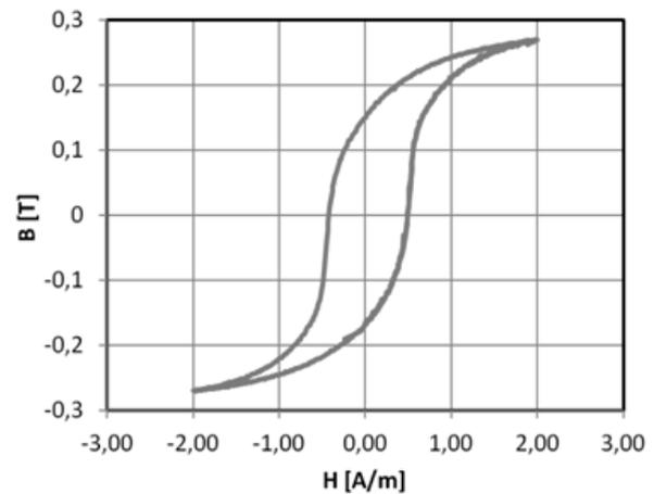
**Fig. 3. Exemplary results of the measured quasi-static hysteresis loop of  $\text{Co}_{67}\text{Fe}_3\text{Cr}_3\text{B}_{12}\text{Si}_{15}$  alloy. Note the extraordinarily low coercive force of the material**
