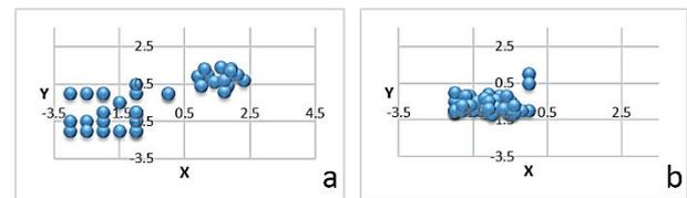
Test 2: repeatability at placing position.
