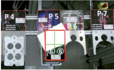
**Fig. 18. Label recognition with partial occlusion**
