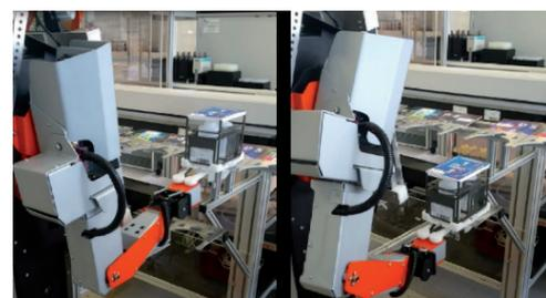
**Fig. 17. Grasping operation for the required labware**
