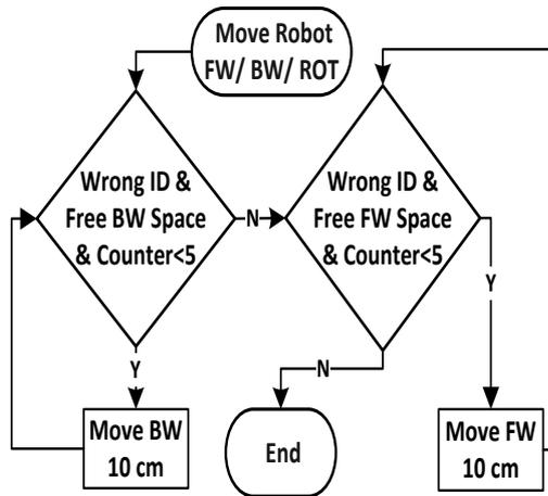
Fig. 8. ID reading correction by movement
