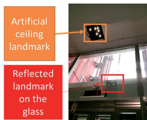
Fig. 7. Reflective ceiling landmark on the glassy wall
