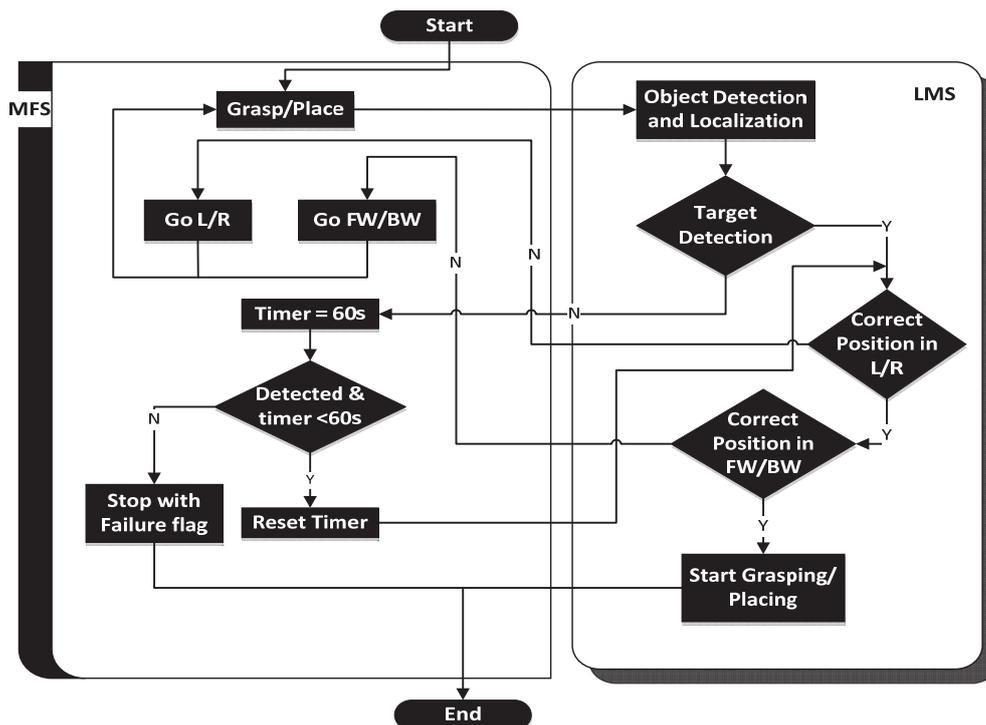
Fig. 32. Operation processes of the position correction in front of (Grasping/Placing) station
