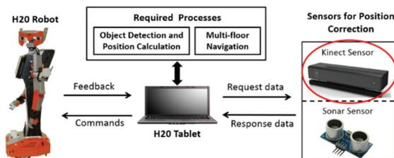
**Fig. 25. System architecture of robot pose correction**
