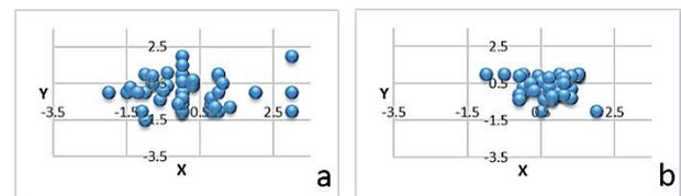
Test 3: repeatability at robot charging position.
