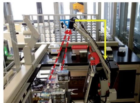
**Fig. 30. Position calculation and extrinsic calibration**
