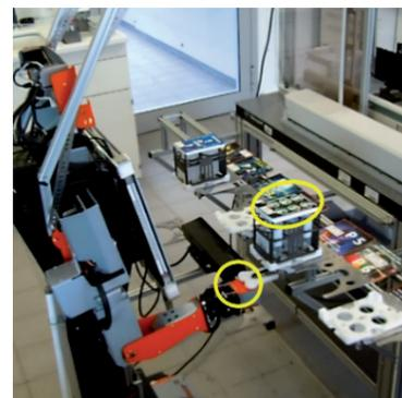
**Fig. 21. End effector tracking in grasping task**
