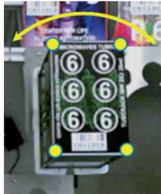
Fig. 22. Orientation angle for labware manipulation
