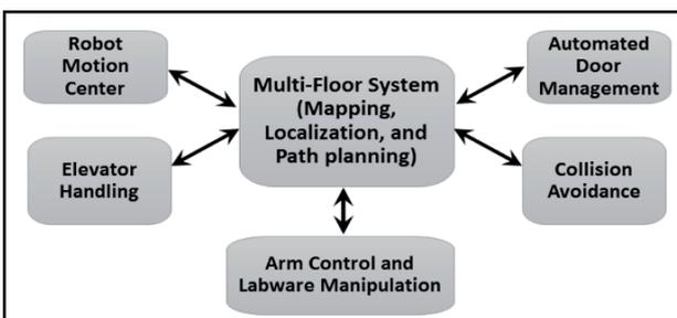
Fig. 3. Main parts of multi-floor transportation system
