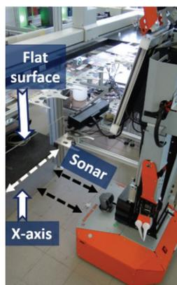
**Fig. 28. Robot pose correction based on sonar sensors**
