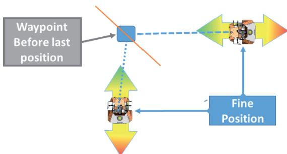
Fig. 23. Fine position correction based on last direction
