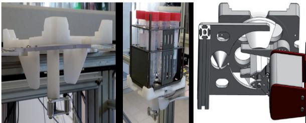
**Fig. 13. Design of gripper and labware container**
