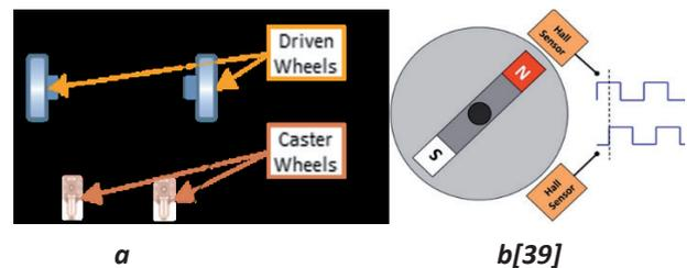
**Fig. 26. a: wheels platform, b: magnetic encoder**
