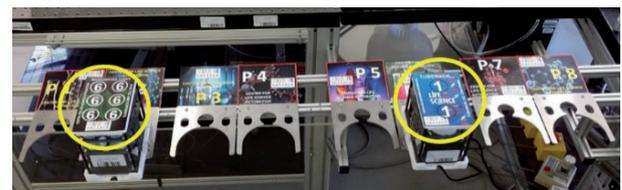
**Fig. 16. Labware label on lid for identification process**
