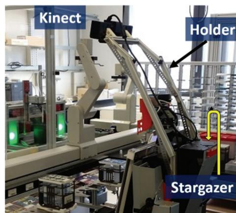
Fig. 11. Kinect holder fixed on the H20 body
