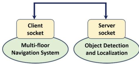
Fig. 31. Client-server model for system integration
