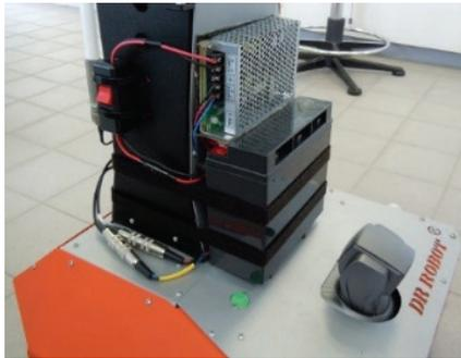
**Fig. 12. Battery and stabilizer for Kinect sensor**
