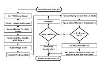
Fig. 20. Internal button detection flowchart
