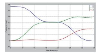
Fig. 31. End effector position versus time
