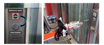
Fig. 16. SURF algorithm with F200 camera for button detection and localization
