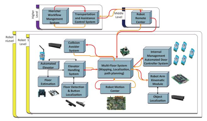
Fig. 2. Complete structure for mobile robot transportation system
