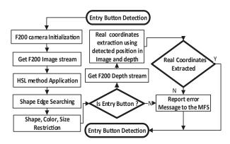
Fig. 14. HSL-based entry button detection
