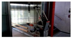
Fig. 29. Left arm configuration to keep the elevator door open
