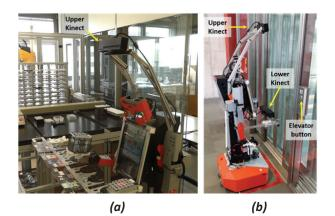
Fig. 3. a) H20 robot in grasping task; b) the H20 robot is in front of the elevator door
