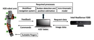
Fig. 6. Architecture of button pressing system
