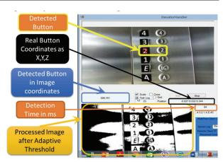
Fig. 21. Elevator handler GUI and Internal button operation
