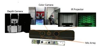
Fig. 5. RealSense F200 camera components
