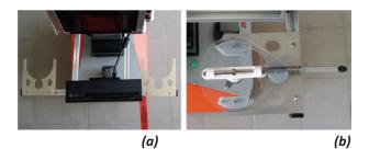
Fig. 11. a) Holder for elevator finger and labware container, b) the elevator finger sits on the holder
