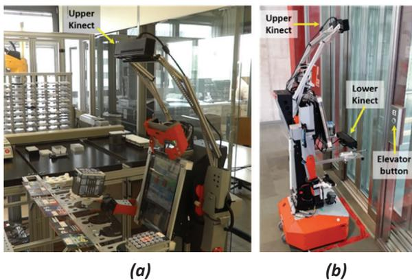
**Fig. 3. a) H20 robot in grasping task; b) the H20 robot is in front of the elevator door**
