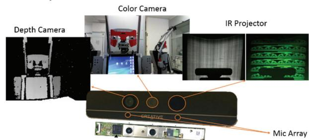
**Fig. 5. RealSense F200 camera components**
