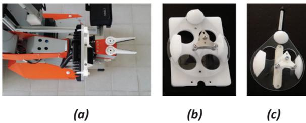
Fig. 9. Design of a) arm gripper, b) labware container bottom, c) button finger bottom
