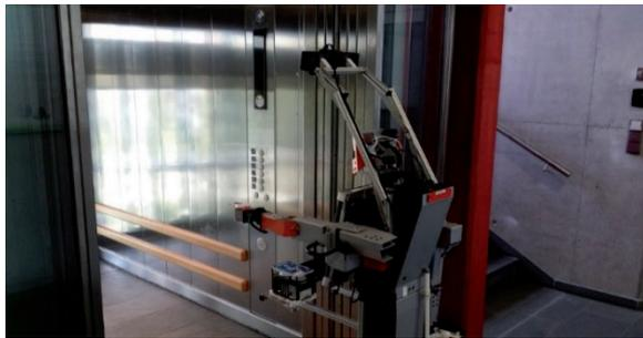
**Fig. 29. Left arm configuration to keep the elevator door open**
