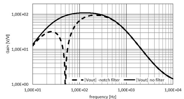
**Fig. 4. Transfer function of filtering part of analog circuit with activated and deactivated 50Hz notch filter**
