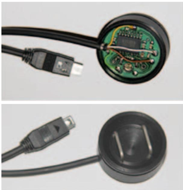
**Fig. 5. Integrated EMG, MMG probe: (a) inner view – EMG front-end circuit, (b) electrode and acoustic chamber view**
