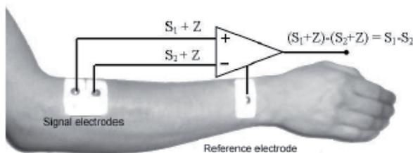
**Fig. 2. The Idea of differential measurement;  $S_1$ ,  $S_2$  – useful signal,  $Z$  – noise**
