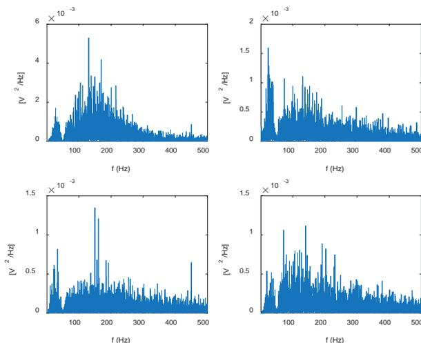
**Fig. 9. Noise power density for relaxed muscles. Energy of the noise are (left to right and down): 0.06; 0.026; 0.017; 0.02 V<sup>2</sup>**
