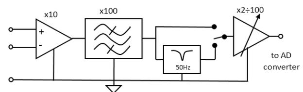
**Fig. 3 Analog part of measurement experimental setup**
