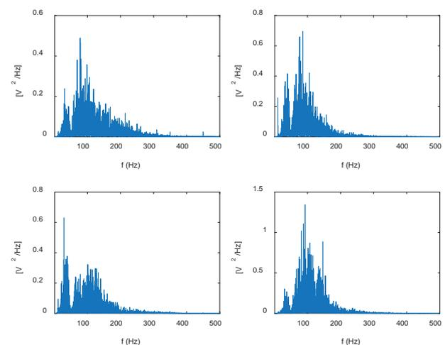
**Fig. 7. Examples of power density EMG signals. Notch filter active. Energy of the signals are (left to right and down): 4.4; 4.9; 4.4; 9.0 V<sup>2</sup>**
