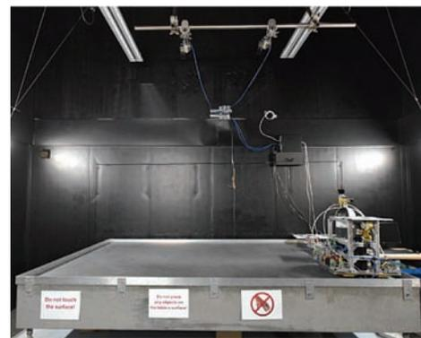
**Fig. 7. The test-bed. 1 – the air bearing table, 2 – the space robot, 3 – the illumination system, 4 – vision system cameras**
