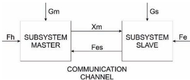
Fig. 3. Block diagram of the presented method with the force-feedback estimation block
