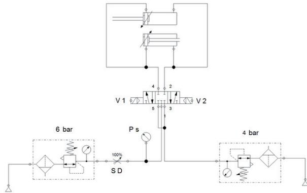
**Fig. 6. Pneumatic scheme of slave**
