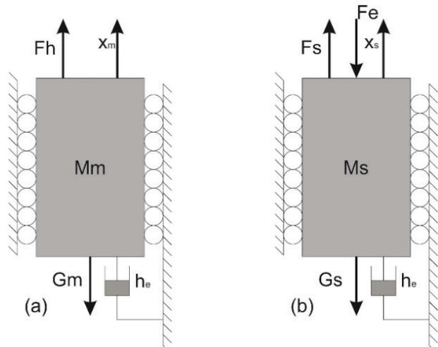
Fig. 1. Graphical presentation of models: master subsystem (a), the slave subsystem (b)
