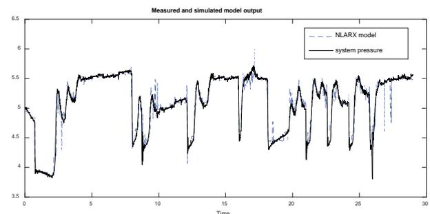
**Fig. 11. NLARX model response against the measured signal**
