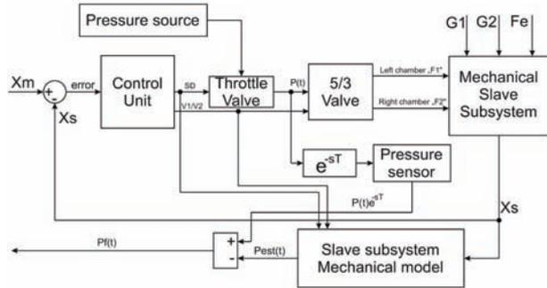
**Fig. 12. Subsystem Slave control unit including delay in the pneumatic tubes**
