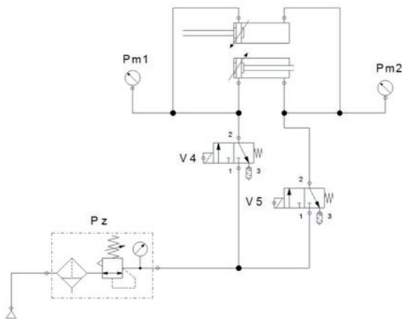
**Fig. 7. Pneumatic scheme of Master**
