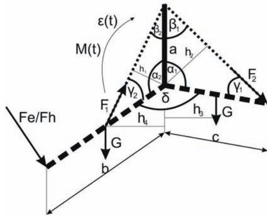
**Fig. 9. The geometrical relationships in manipulator structures considered in inverse modelling**
