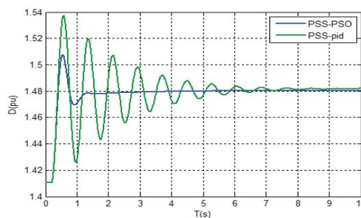
Fig. 5. Functioning system in the nominal regime used of TBB-500 connected to a long line with, PSS-PSO, PSS-PID (Ug, Pe, skid, delta)
