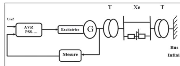
**Fig. 1. Block schematic diagram of the proposed SMIB Power system controller**
