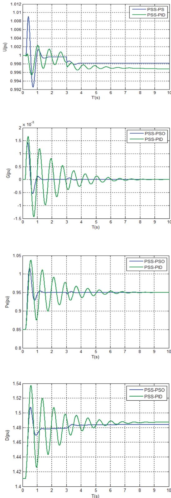
**Fig. 6. Functioning system in the nominal regime used of TBB-500 connected to a long line with, PSS-PSO, PSS-PID (robustness tests) (Ug, Pe, skid, delta)**
