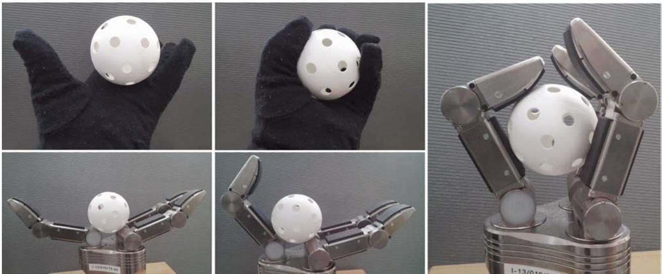
**Fig. 6. Calibration of the spherical grip (from left): hand and gripper open, hand and gripper at the beginning of the calibration process (large discrepancies in the pose of two fingers), spherical grip after calibration**
