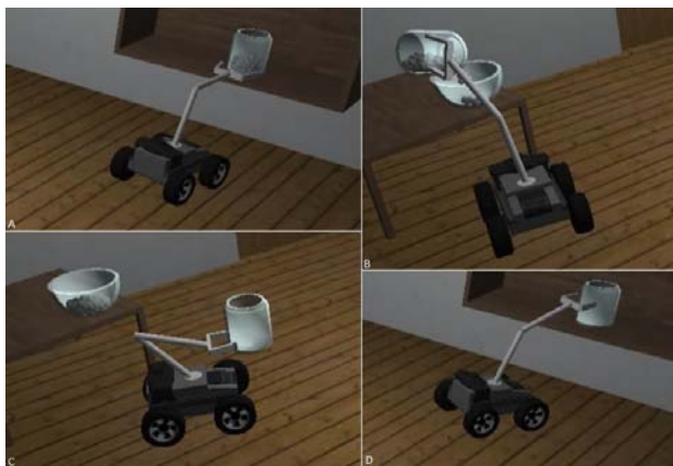
Fig. 5. Realization of the sample task in the simulation environment; a) grabbing the initial object, b) turning the robot arm over the final object, c) driving to the original location of the initial object, d) returning the initial object to its original position.
