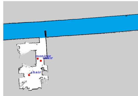
**Fig. 7. Grid-based map of the environment and recognized objects**
