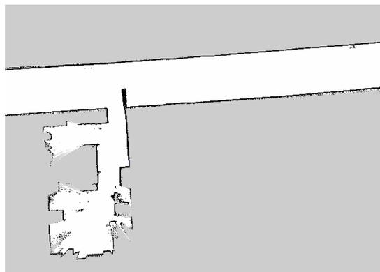
**Fig. 3. Grid-based map of the environment**
