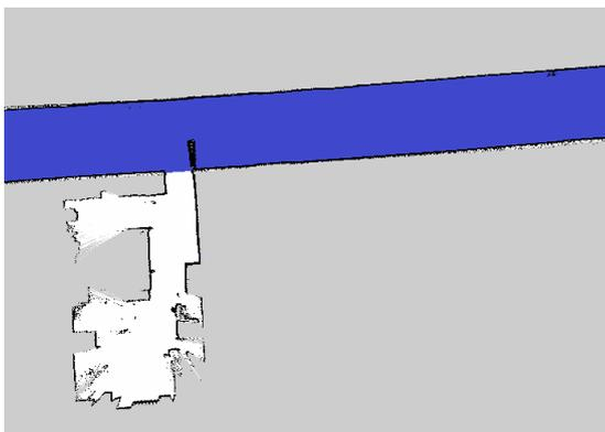
**Fig. 6. Grid-based map of the environment and place classification: blue – corridor, black – obstacles**
