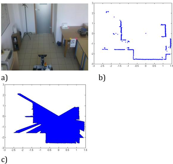
**Fig. 5. Data obtained by the laser range finder: a – the image of the laboratory, b – a scan taken in the laboratory, c – polygonal approximation of the scan**
