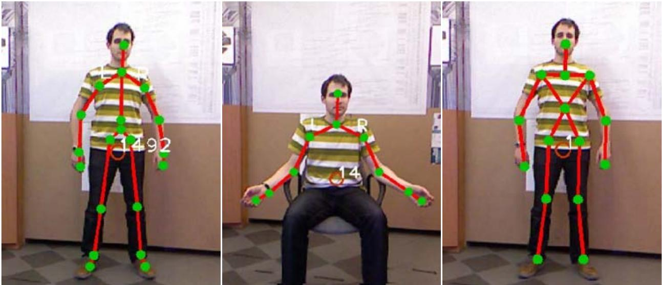
**Fig. 2.** Comparison of detected silhouettes (starting from the left: Kinect SDK, Kinect SDK "Seated mode", OpenNI/NiTE)
