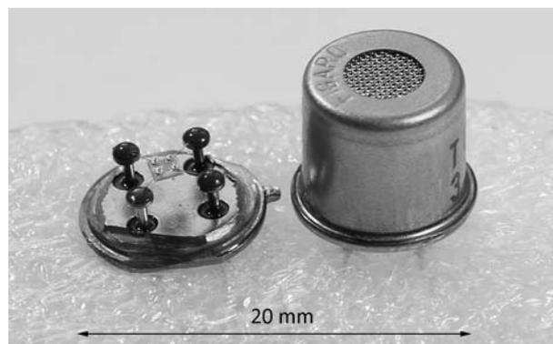
**Fig. 1. Commercial Figaro TGS 2620 Gas Sensor with and Without Cover**
