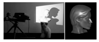
Due to that one can obtain different measurement values, closeness and measurement times adapted to the particular object. The measurement is based on the optical methods, which make possible synchronous canvassing of the object's preferred orientation. Formulated system can be used in technology, medicine or for making archives and documentation of the works of art.
