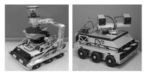
A laboratory mobile robot Electron is been con-structed at the Warsaw University of Technology, as a common project of two Institutes: Automation & Robotics, and Automation and Applied Informatics. Four constructed prototypes can perform team tasks. The robots are autonomous units; they all have independent control systems and communication modules.
