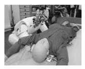
An advanced sensors system of that robot is composed from over 1800 touch sensors. For the sake of safety the robot is provided with smaller and weak engines. However, thanks to intelligent control and many sensors, 155-cmhigh robot is able to lift easily, for example, 30-kg weight package from a table or 66-kg from the bed.
