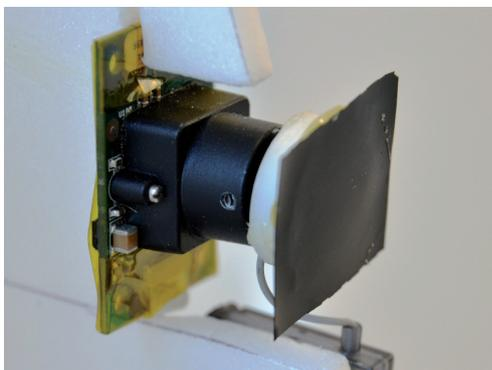
**Fig. 4. CMOS camera with daylight blocking filter**
