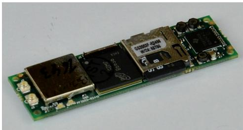
**Fig. 5. Gumstix Overo Firestorm computer on module**
