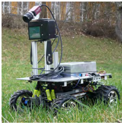
Figure 4. Robot with mounted 3D laser ranging sensor
