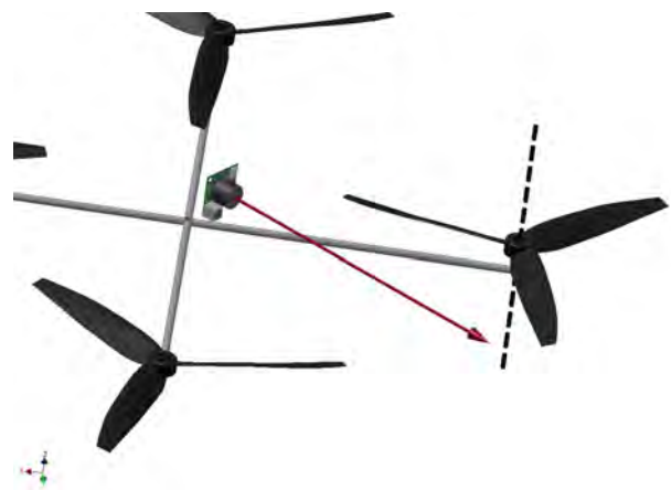
Fig. 1. Sensor in a plane parallel to the axis of rotation of the propeller
