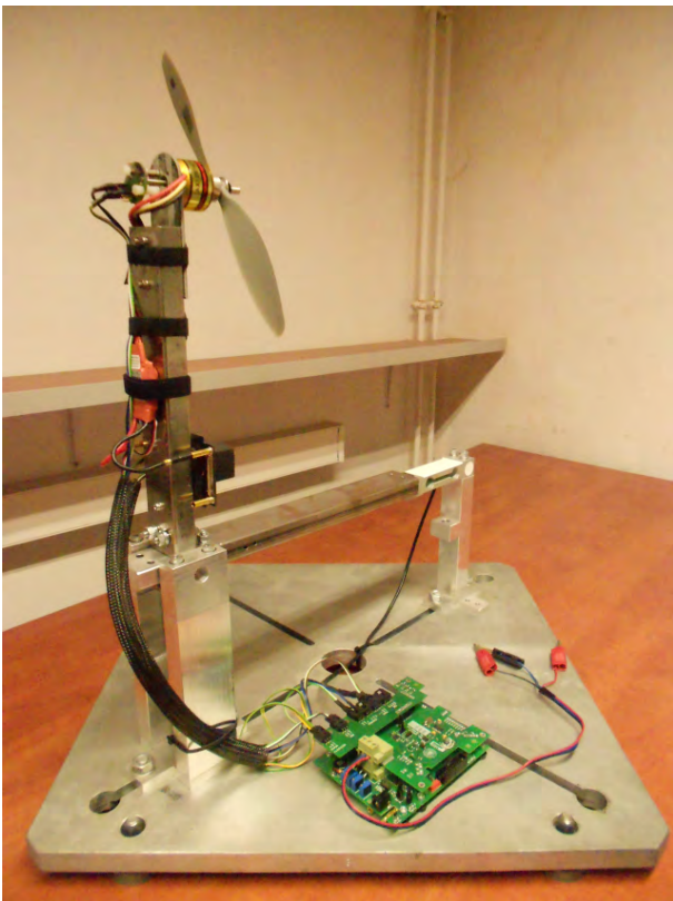
Fig. 3. Dynamometer with drive unit and the propeller
