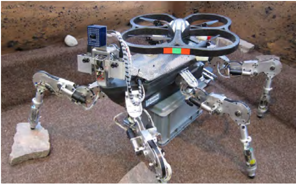
Fig. 3. ARDrone landed on the back of LAURON IVc. Vital energy can be saved for the next assignment
