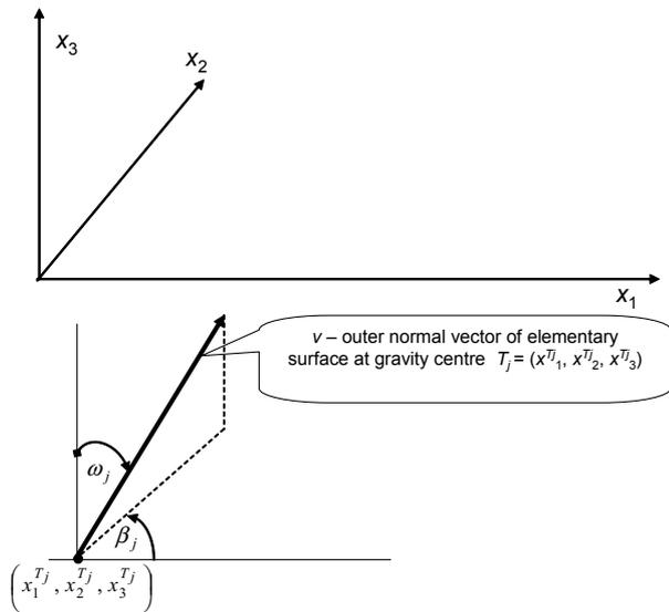
Fig. 2. Parameters determining the elementary surface  $p_j$
