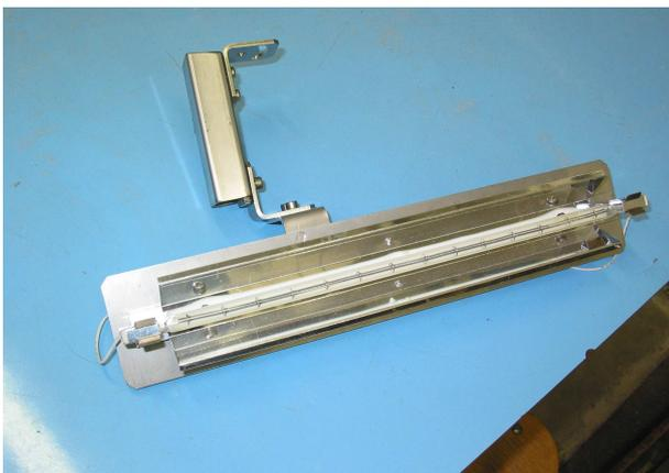
Fig. 1. Philips infra heater with 1000W capacity
