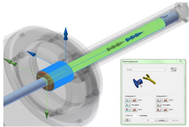
Fig. 4. Selection of components of screw gear
