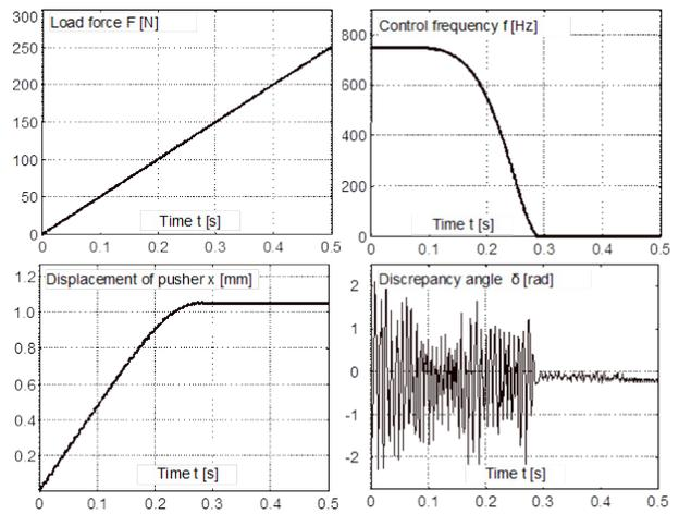
Fig. 9. Results of simulation of a linear actuator driven by stepping motor
