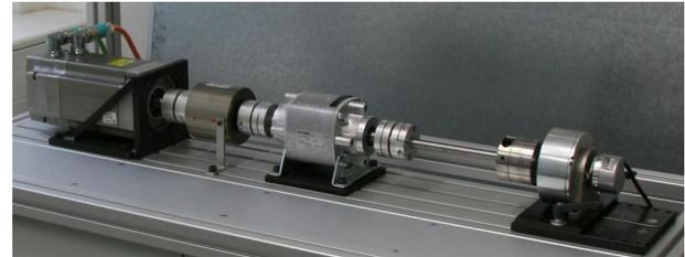
Fig. 3. Test rig with known moment of inertia
