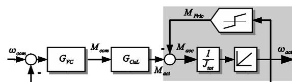
Fig. 2. Scheme of the velocity loop [9] with:
