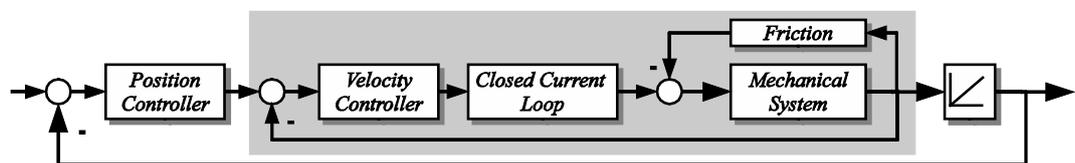
Fig. 1. Cascaded position control with velocity loop (grey)
