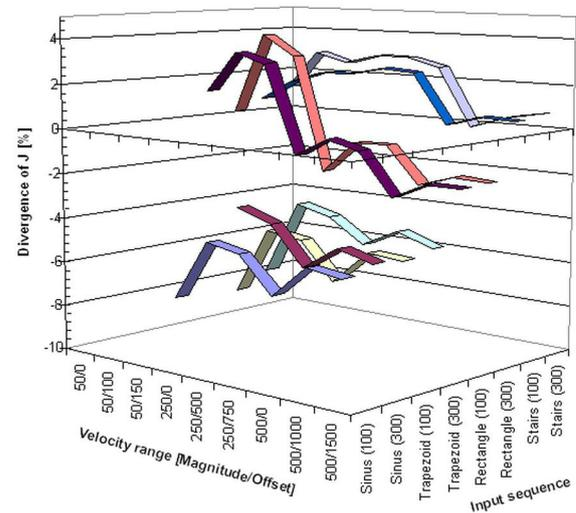
Fig. 4. Identification results for the moment of inertia  $J_{tot}$  with velocity controller setting 1
