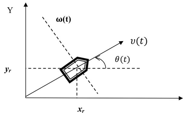
Fig. 1. Geometry of the robot motion on the Cartesian plane
