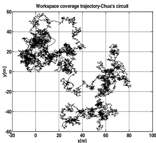
Fig. 7. Workspace coverage trajectory of the chaotic mobile robot, Chua's circuit
