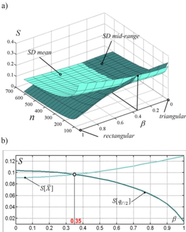
Fig. 1. Efficiency of single component sample estimators of  $Trap(a,b)$  distributions [10]: a. Dependences of sample mean and midrange standard deviations  $S$  on ratio  $\beta$  of linear trapeze bases and of sample size  $n$ , b. cut-set of  $S$  surfaces for  $n=const.=400$
