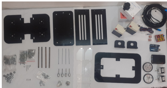
Figure 1. Robot components used in the proposed mobile robot platform
