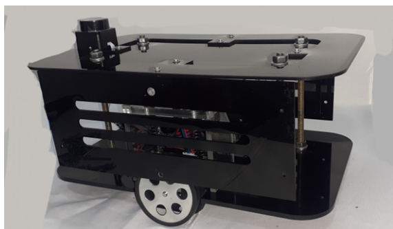
Figure 2. Fully assembled differential-drive mobile robot system
