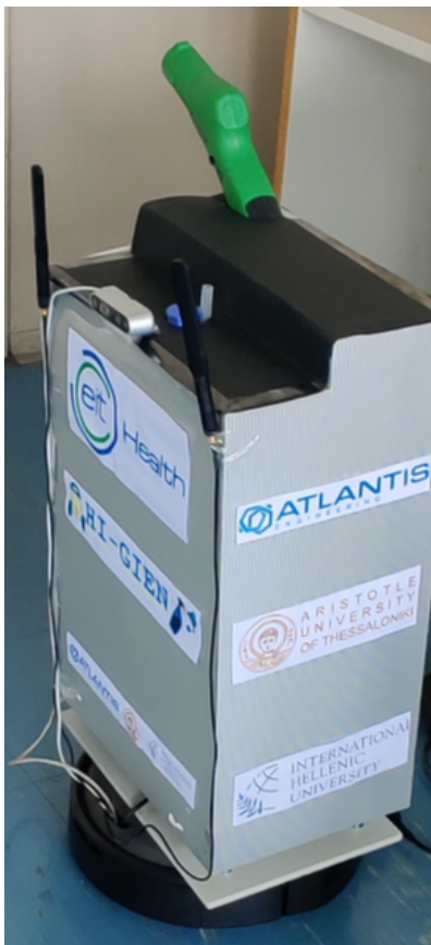
Figure 1. The robot chassis consists of the robotic vehicle base station and a high-top frame for mounting the depth camera and the disinfection electrostatic sprayer. A depth camera is mounted on top of the frame, and a disinfection subsystem is mounted inside the frame, culminating in the spray nozzle
