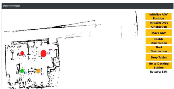
Figure 9. Following a two-hour inspection, the locations identified requiring further investigation were marked on the diagram. The circles' color represents the risk level associated with each area. In contrast, the size of the circles indicates the extent of the area in which human movements were observed
