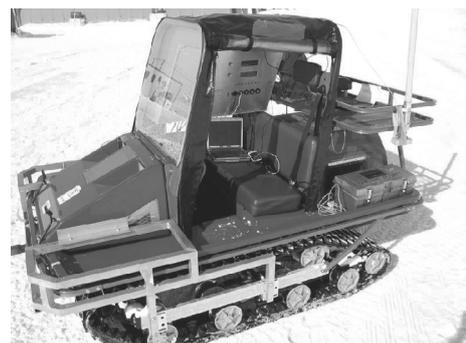
Fig. 2. The MARVIN II polar robot in Antarctica in 2006, used to autonomously gather radar data of ice sheets.
