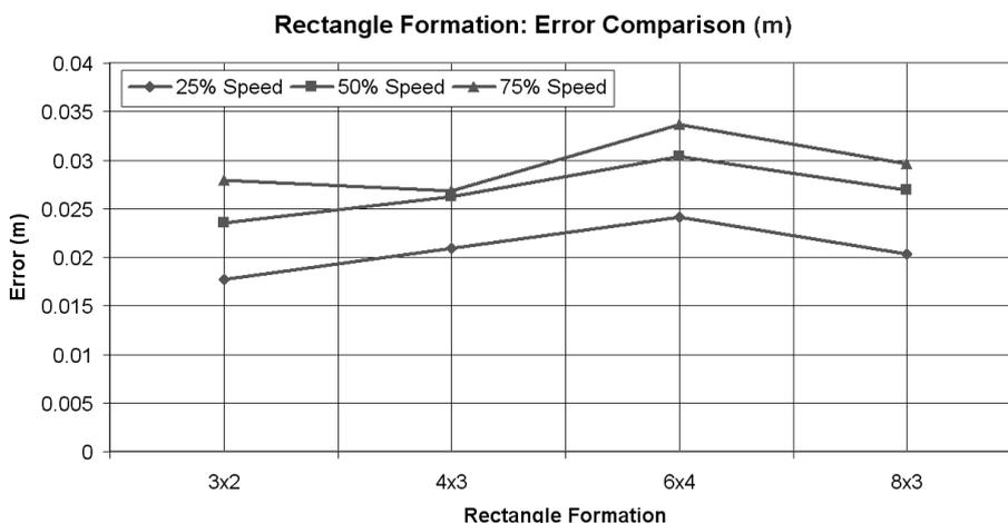
Fig. 14. Rectangular Grid: Error Versus Speed Comparison.
