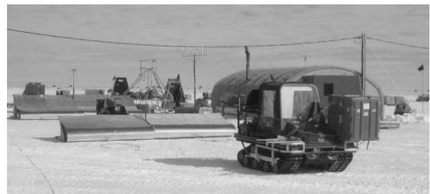
Fig. 3. MARVIN II polar robot preparing for a bi-static radar experiment.
