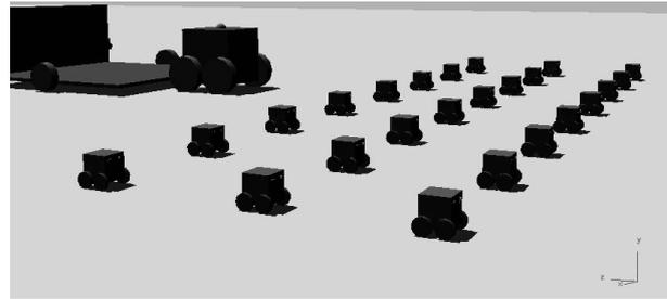
Fig. 9. Simulation images of completed robot seismic grids, demonstrating abilities to form various shapes of various spacings.
