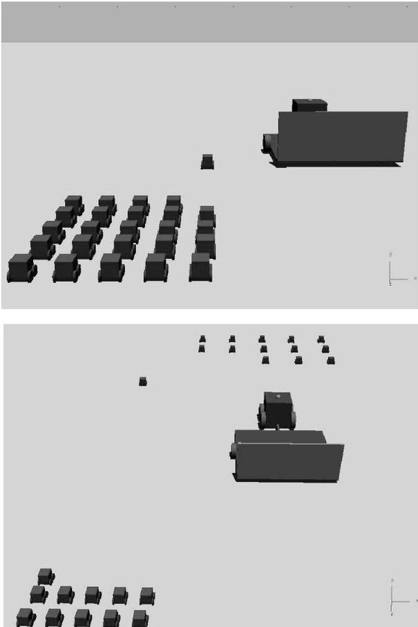
Fig. 8. Simulation images showing a team of mobile robots forming a square seismic grid, one-by-one from top-right to bottom-left.
