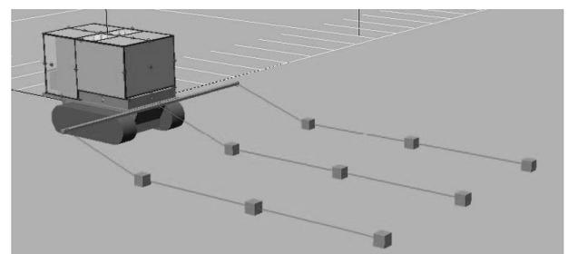
Fig. 5. Simulation image of an autonomous robot towing a three-streamer array, used for studying towing of streamers and how turning affects strain of the towing structure and travel of the streamer components.
