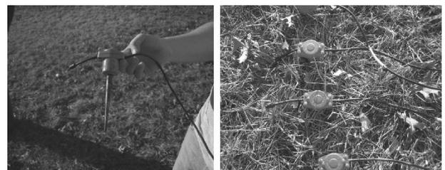
Fig. 1. Conventional spiked geophone (left) and several deployed by inserting the spikes into the surface (right).
