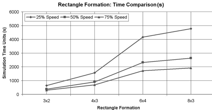
Fig. 11. Rectangular Grid: Formation Time Versus Speed Comparison.
