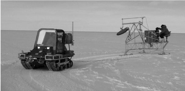
Fig. 4. CReSIS MARVIN II polar robot turning while pulling a radar apparatus.
