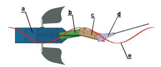
Fig. 2. Motion of the proposed mechanism, a) the first segment the head, b) the second segment, c) the third segment, d) the fourth segment and the caudal fin, e) superimposed image of sinusoid.
