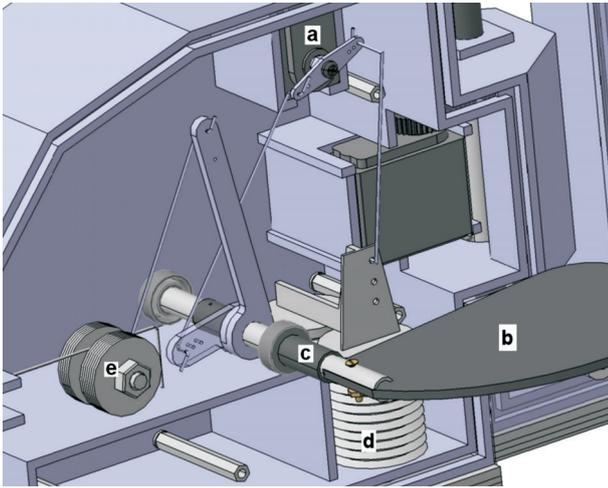
Fig. 4. Diving mechanism, a) servo, b) pectoral fin, c) pectoral fin's axis, d) two silicon tubes, e) additional weight.
