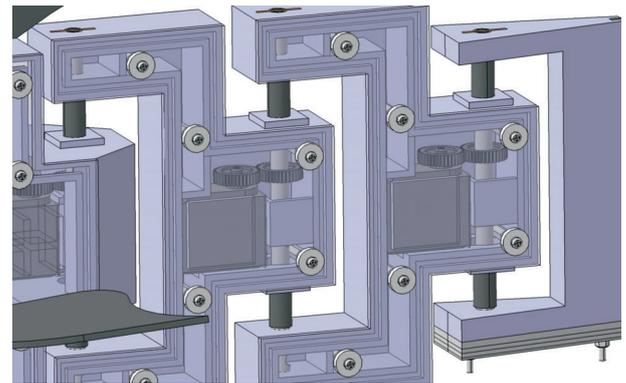
Fig. 3. The transmission of the second and the third segment.
