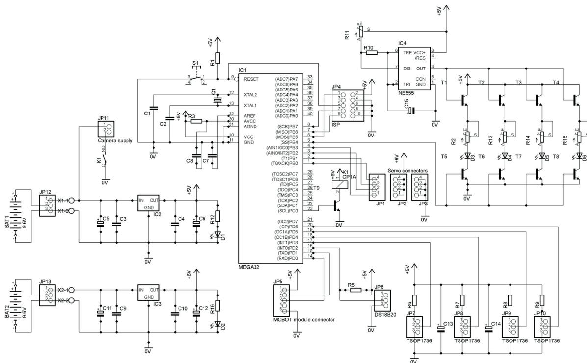
Fig. 6. The complete scheme of the robot's electronic control board.
