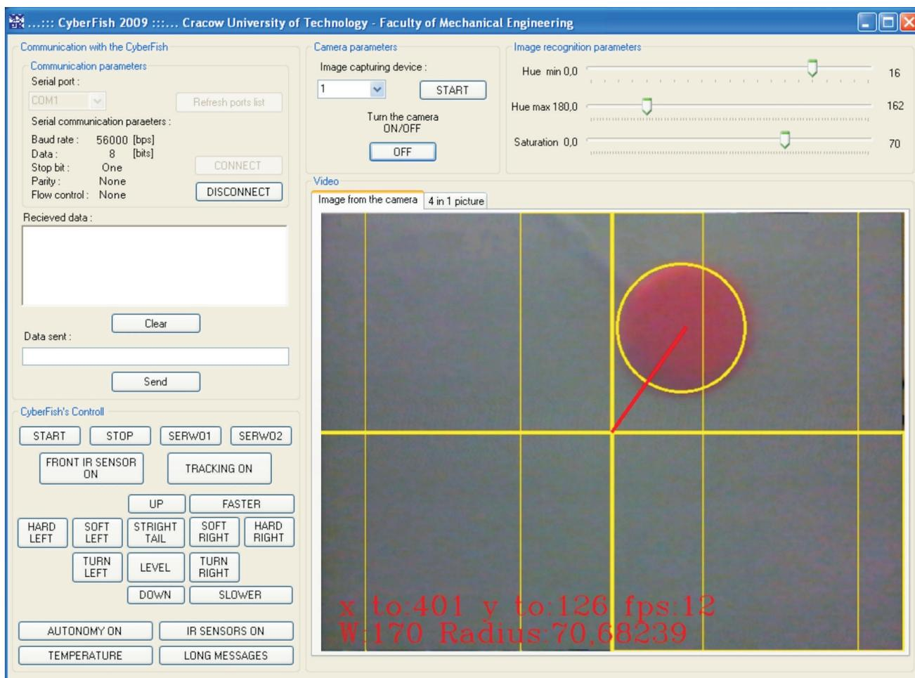
Fig. 7. The robot's control application window.
