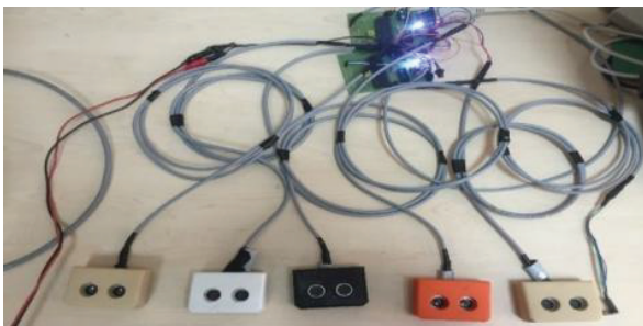
Figure 32. The version operated with improved detection cards for calipers and ultrasonic sensors
