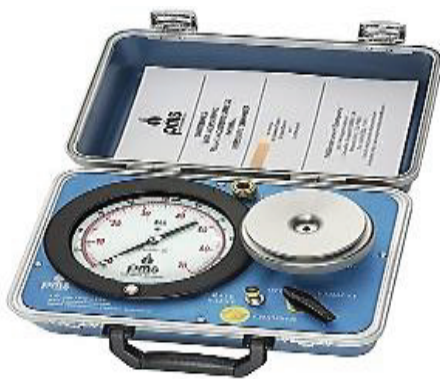
Figure 21. A portable Scholander Pressure Chamber
